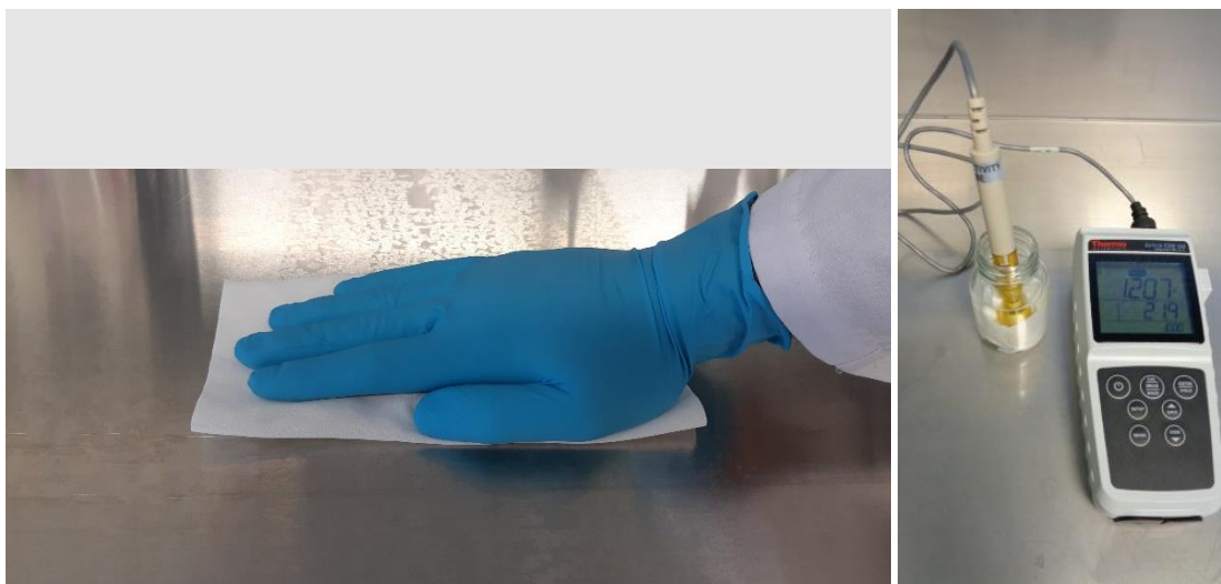
Picture 2: Photo of sample collection via wiping of the surface with a wetted wipe and subsequent measurement of the residues from the wipe in aqueous solution using a Conductivity meter.
