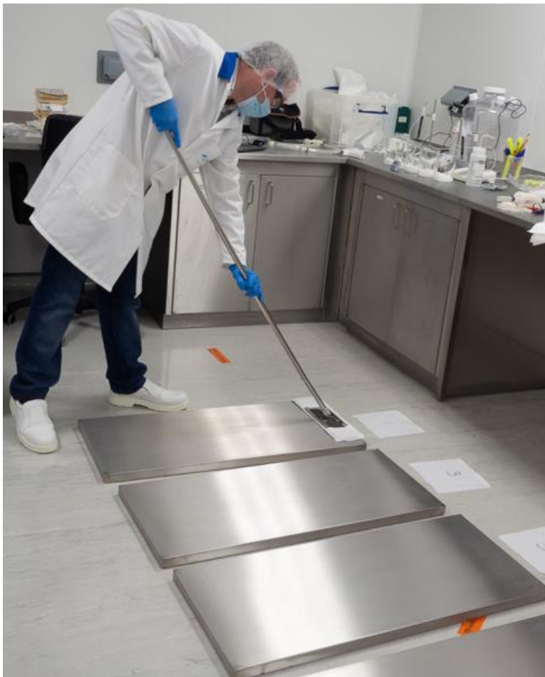
Picture 4: Application of disinfectant via mopping on stainless steel panels.
